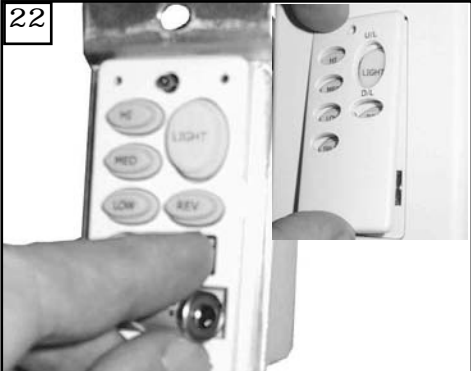
22 Remove cover by snapping off from top or bottom. Install 12V battery into wall remote. Duracell MN21 / Eveready A23 / GP 23A all 12V.
